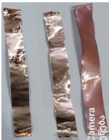
Fig. 2. Typical graphite layers obtained experimentally
