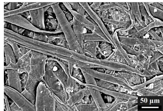
Fig. A1. SEM image of the paper surface at 270x magnification.
